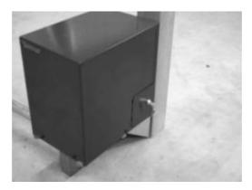
• Turn knurled disc anticlockwise for arm to be released from gearbox.
